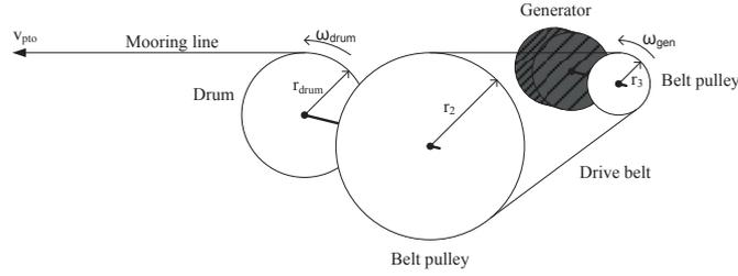
Figure 2.1: Illustration of the linear to rotational gear ratio
