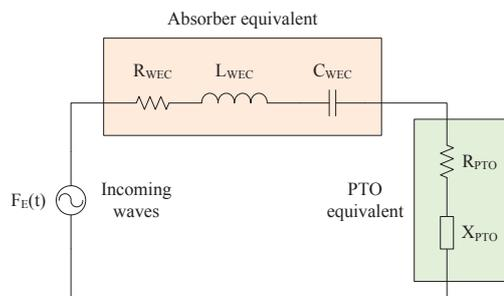
Figure 2.15: Equivalent circuit for Wave Energy Converter and Power Take Off
