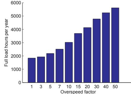
Figure 2.13: Annual load hours with different overspeed ratios
