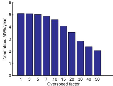
Figure 2.12: Annual energy production with different overspeed ratios
