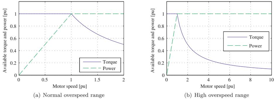
Figure 2.10: Ideal torque and power curves for PMSM
