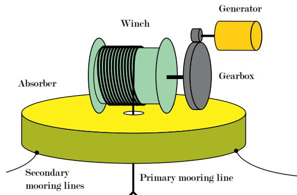
Figure 2.3: Principal sketch of the PTO and WEC
